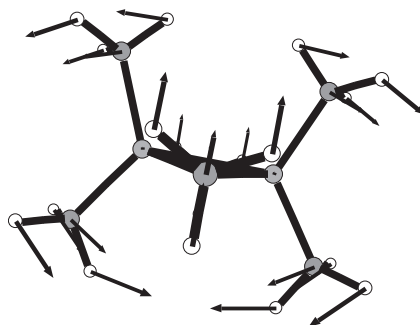
Figure 5. The minimum-energy configuration of \text{Al}_2(\text{CH}_3)_6 . The arrows indicate a bend mode of the whole molecule, about the bridging methyl groups. This mode has the absolutely lowest energy.
